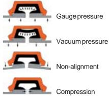
The standard gasket made from EPDM rubber is suitable for all substances including many chemical compounds. Working temperatures range from -35 to +110°C. A nitrile or silicon gasket is recommended if there is long-term contact with petroleum products.
