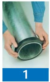
The gaskets outer mating surface and the lips' inner mating surfaces are lightly greased with a lithium or silicon-based grease. The rubber gasket is slid onto one of the pipe ends.
