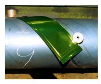
X-ray inspection of a weld joint
