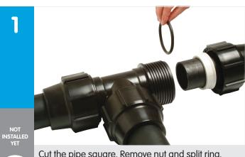
Cut the pipe square. Remove nut and split ring. Reposition nut, bush and O-ring on pipe 2x diameters back. Lubricate pipe and O-ring.
