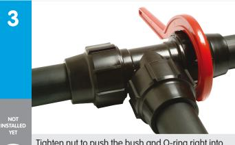
Tighten nut to push the bush and O-ring right into the fitting until the bush is flush with fitting mouth.
