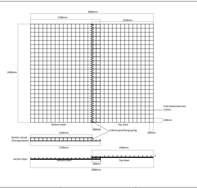
Min tensile strength cross wire 400 MPa Max tensile strength cross wire 500 MPa 400 MPa Min tensile strength main wire Max tensile strength main wire 600 MPa Min weld shear\* 9.3kN Min torque value 18Nm Min penetration 10% Average Zinc coating 100g/m2
